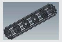
The specially designed packer type rollers used in Hisarlar brand 9-shank cultivators are 550 mm in diameter and are reinforced with 6 intermediate support plates. 1040 alloy 45 mm diameter shredder gears mounted on discs on the shaft are made of 8 mm thick steel.
