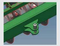
Goble disc harrows have a rear draw bar linkage point. It is also possible to connect other wheeled equipment to the rear of the machine on the road. (roller group, etc)
