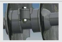
The disc bearing housings of disc harrows are maintenance-free, lubrication-free bearings.
