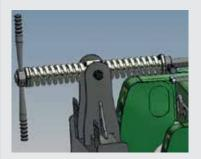
It is possible to change the angle of the draw bar and the penetration depth by means of the adjustment lever in goble disc harrows.
