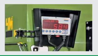
With the optional high quality and accurate weighing system, it is easy to calculate feed consumption.
