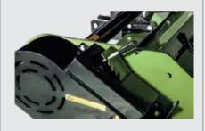
It is possible to easily adjust the belt tension with the belt pulley adjustment lever located on the side of the mulchers.
