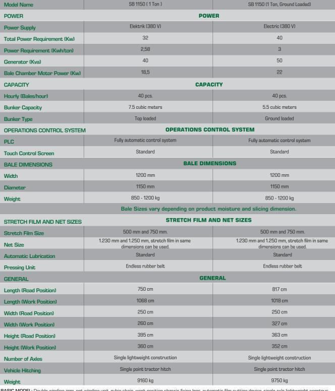
Silage Packing Machine (1 Ton)
