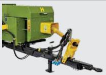
Hydraulic road-work position; Controlled from the cab via hydraulic joysticks, the road-work position adjustment provides comfort and easy operation.
